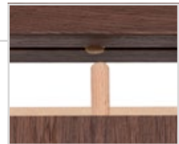
Solid tenon connections
