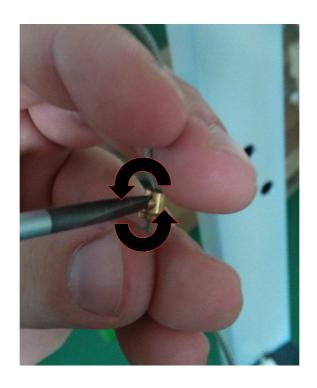
Adjust position of the limiter, in this case move limiter up.
